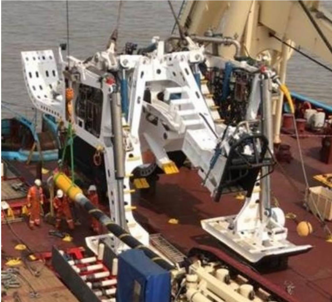
Plate 6.13 Plough which was used to install the offshore export cables at the East Anglia ONE project
