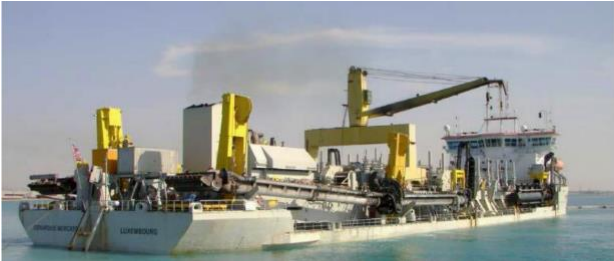
Plate 6.12 Example of a trailer hopper suction dredger (THSD)
